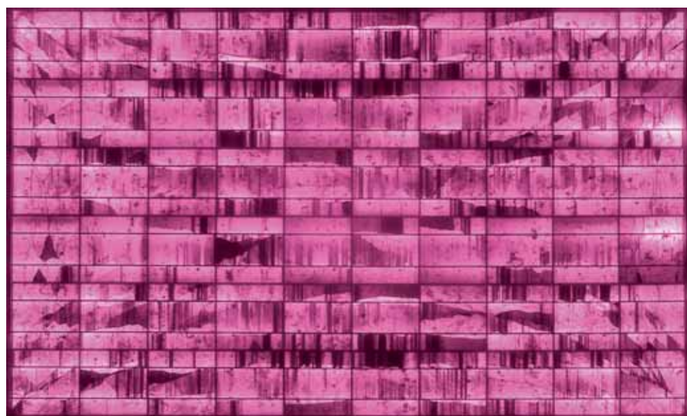
EL imaging from mobile testing highlights inactive cell areas in modules in the field
