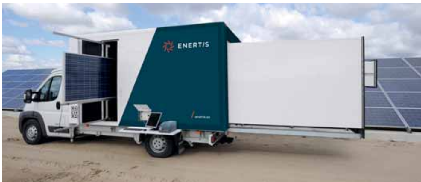
Figure 2. Enertis' PV Mobile Lab.
