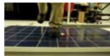
Figure 1. The top, middle and bottom pictures show the loading set-up for Tests 1, 2 and 3 respectively. The local bending of the module is measured by a laser distance measurement close to the loading point (black box in the images).
